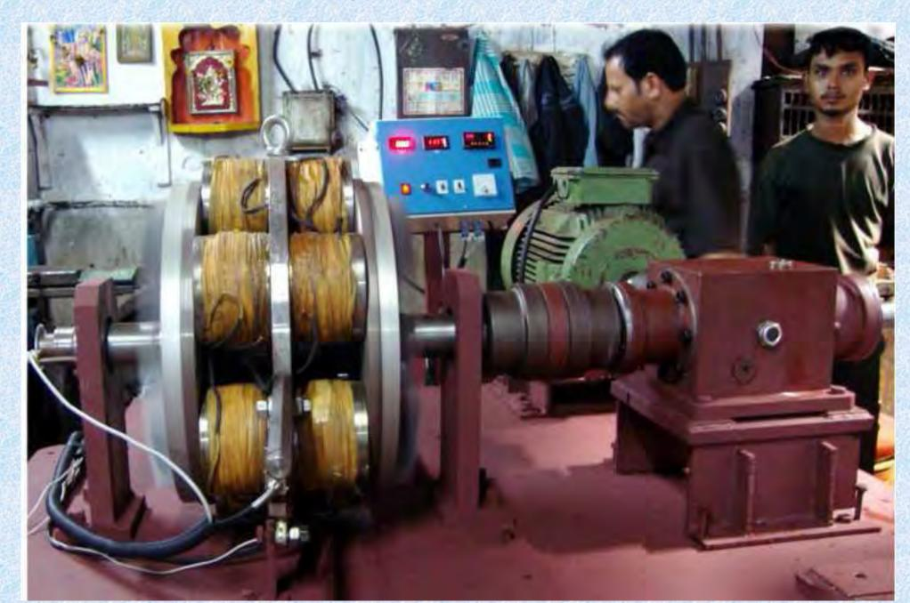
Our Proprietary APPSYS MOTOR TEST/ GEAR BOX TEST software developed for motor test to monitor & display Motor Input Power, Output Power, Efficiency, Input Voltage, Motor No Load Current, Full Load Current, No Load & Full Load Speed, No Load & Full Load Torque, Power factor, Motor temperature, bearing temperature, winding temperature.
